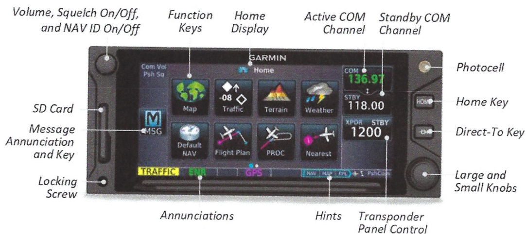
Figure 2 - GTN 635Xi/650Xi Control and Display Layout
