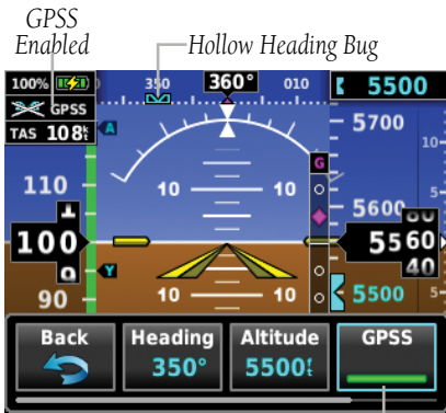
Figure 4-3 GPSS Enabled - PFD
