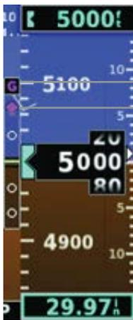
Figure 2-25 Vertical Deviation Indicator (Glidepath GPS Source) - PFD
