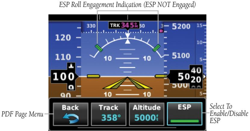
Figure 3-25 AFCS (ESP Enabled)
