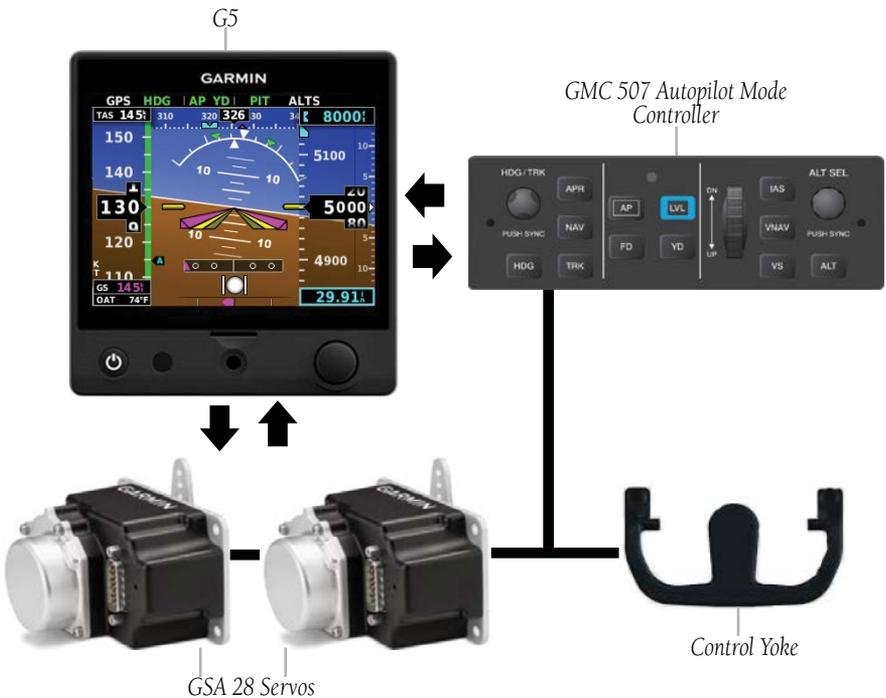
Figure 3-1 Core GFC 500 System
