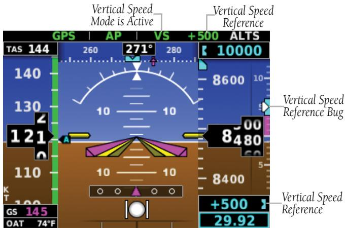
Figure 3-11 Vertical Speed Reference on PFD Page
