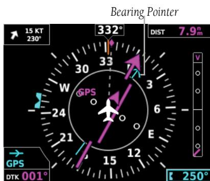
Figure 2-16 GPS Source Bearing Pointer
