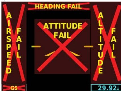
Figure 1-2 G5 PFD Page Failure Annunciations
