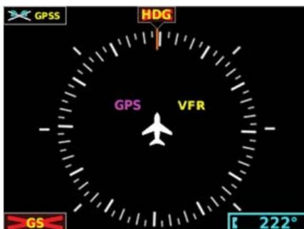
Figure 1-3 G5 HSI Page Failure Annunciations
