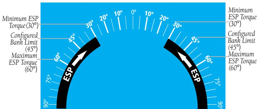
Figure 3-28 ESP Roll Operating Range When Engaged
