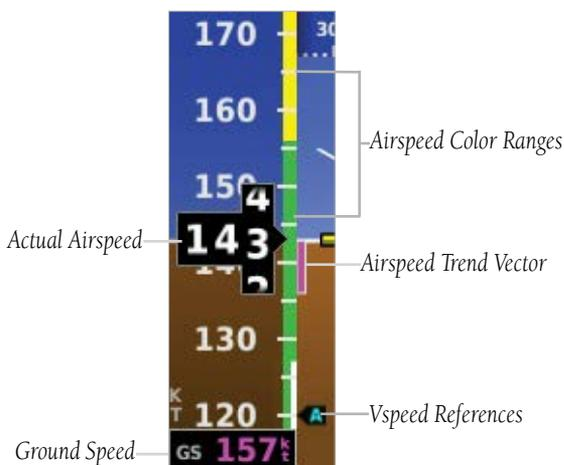
Figure 2-2 Airspeed Indicator
