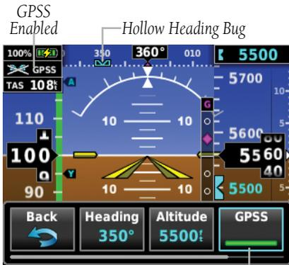
Figure 4-3 GPSS Enabled - PFD
