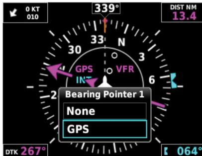
Figure 2-20 Bearing Pointer Source Options
