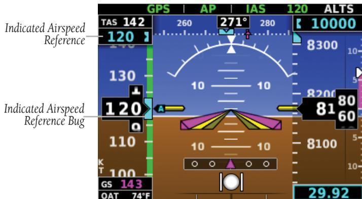
Figure 3-13 Indicated Airspeed Reference on PFD Page
