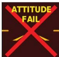
Figure 1-6 Attitude Failure Indication
