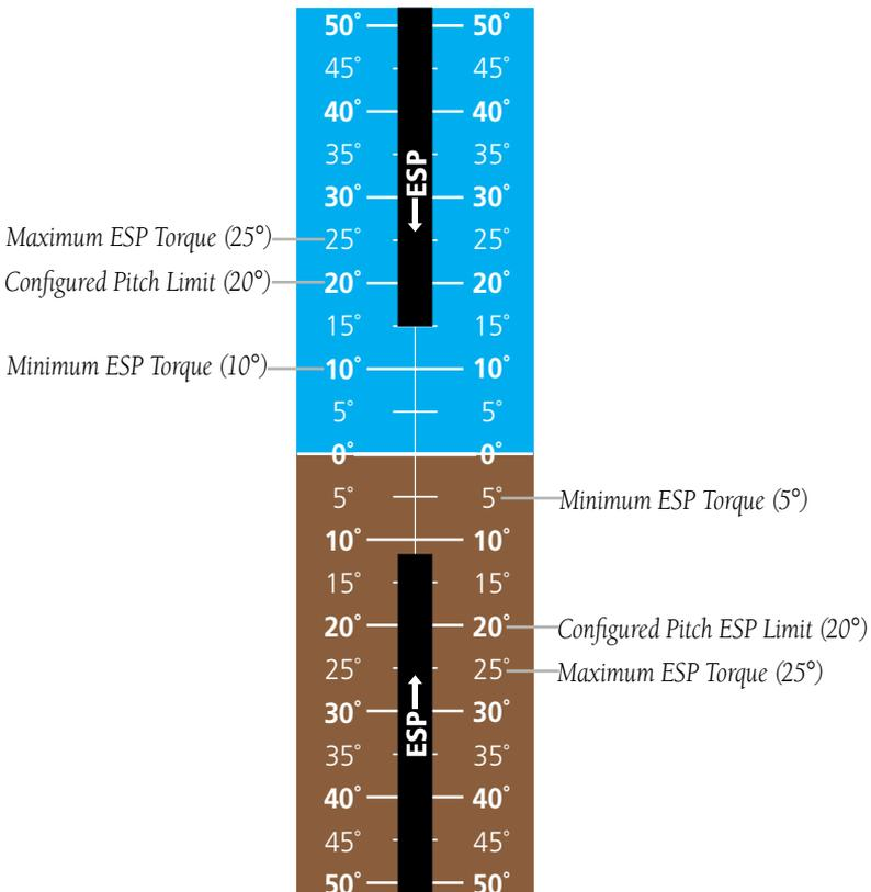
**Figure 3-29 ESP Pitch Operating Range When Engaged**
