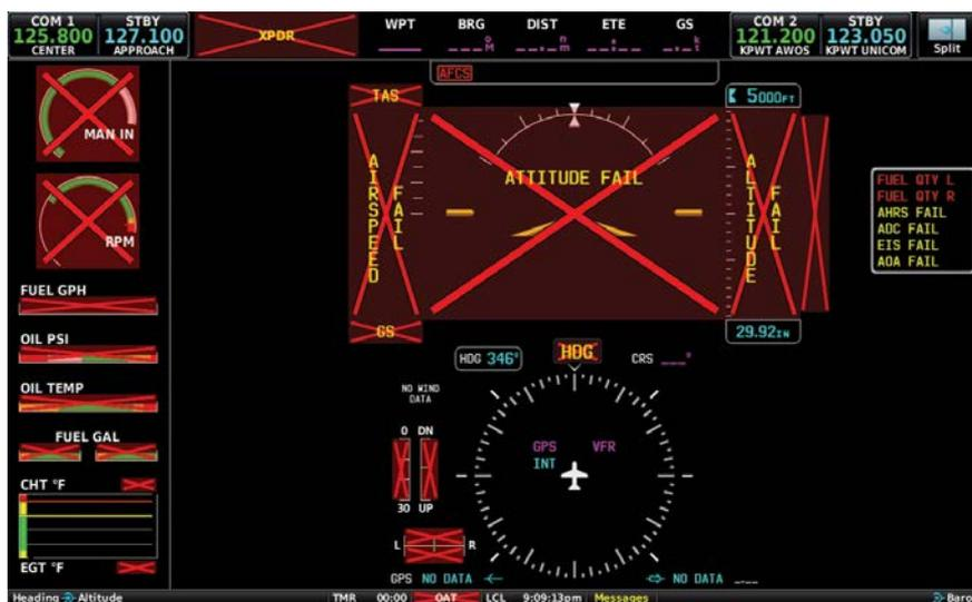
G3X Touch System Failure Annunciations
