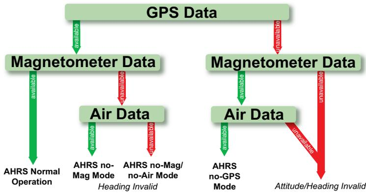
Loss of GPS, magnetometer, or air data inputs is communicated to the pilot by message advisory alerts. Any failure of the internal AHRS inertial sensors results in loss of attitude and heading information (indicated by red 'X' flags over the corresponding flight instruments). If the G3X Touch senses the magnetic heading measurement is valid, but possibly outside of the internal accuracy limits, the numeric heading value on the PFD is displayed in yellow.
