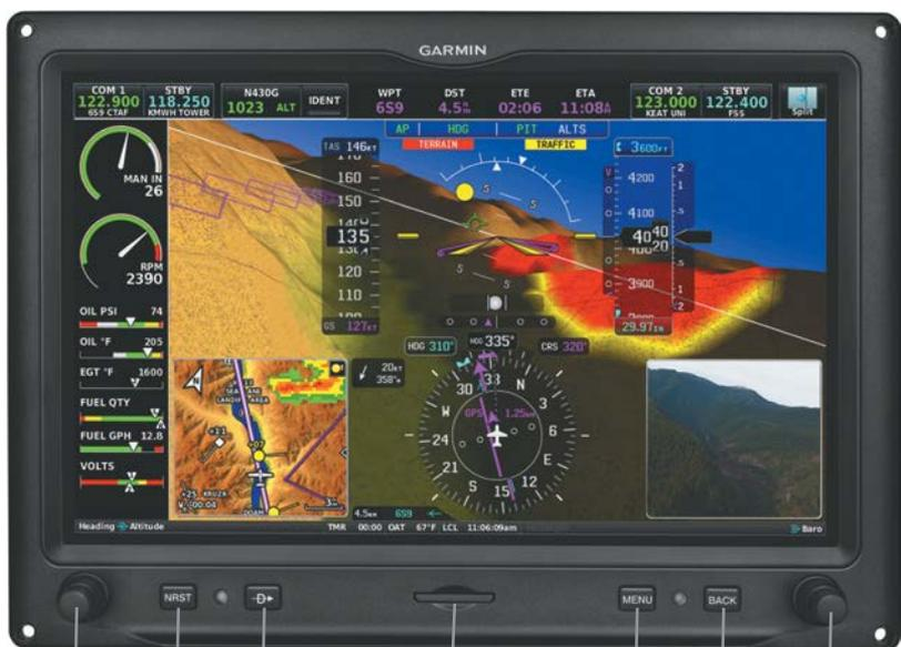
Left Knob    Nearest Button    Direct-to Button    SD Card Slot    Menu Button    Back Button    Right Knob
