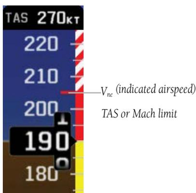
V<sub>ne</sub> Adjusted for True Airspeed
