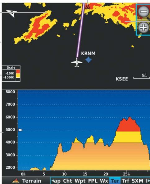
Red Terrain is above the aircraft, or within 100 ft below the aircraft.
