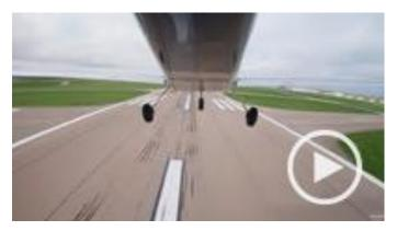
A bounced or firm landing is typically not a hard landing. So, what is a hard landing? It happens when an airplane stalls or drops onto the runway with too high a vertical speed, resulting in damage to the aircraft. It's not just the landing gear that takes the hit—structural damage also extends to the firewall and engine mount, fuselage skin, wings, and so on. See the video...
