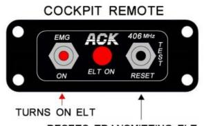
RESETS TRANSMITTING ELT TO THE ARMED MODE PREFORMS SELF TEST WHEN PRESSED WHEN ELT IS IN ARMED MODE the panel. In the cases where they have been inadvertently set off, they are close to the throttle or mixture controls.
