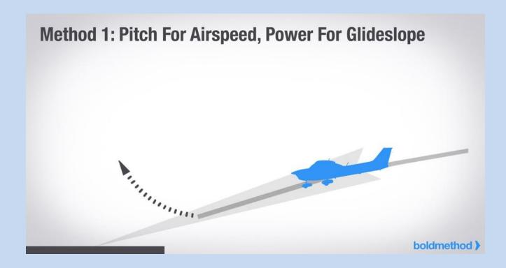
Elevator trim keeps the aerodynamic forces acting on your elevator constant. And since a constant indicated airspeed creates a constant aerodynamic force on the tail, elevator trim will vary your pitch to hold that airspeed.
