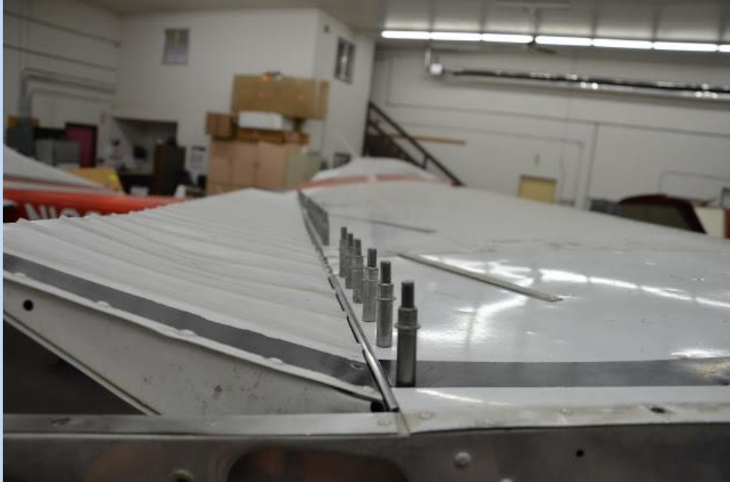
Cleco's on the new Aileron Gap Seals Provided with the Sportsman STOL
