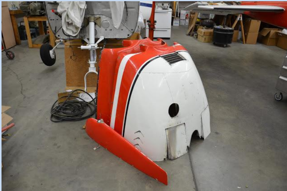
Top and Bottom Cowling (Note the Shark Gill Vents in the Lower Cowling) Wingtips will be replaced with wingtips provided with the STOL kit.
