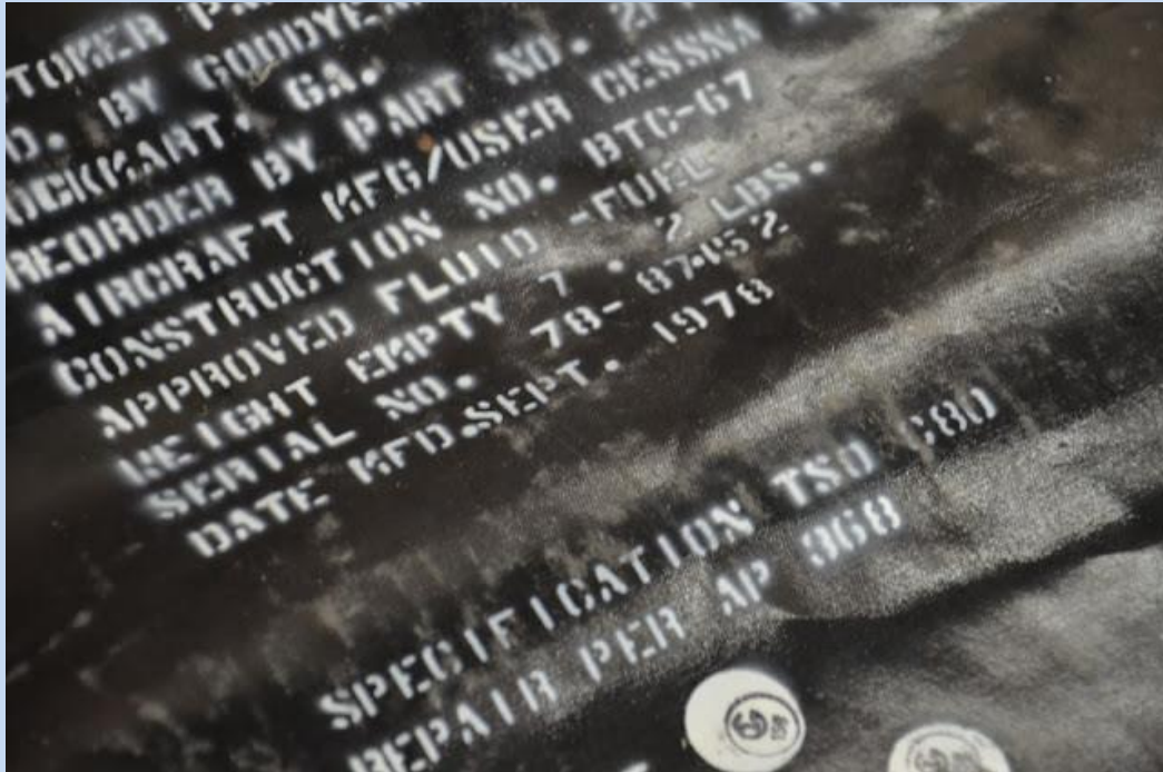
This fuel bladder is from 1978 and needed to be Replaced
