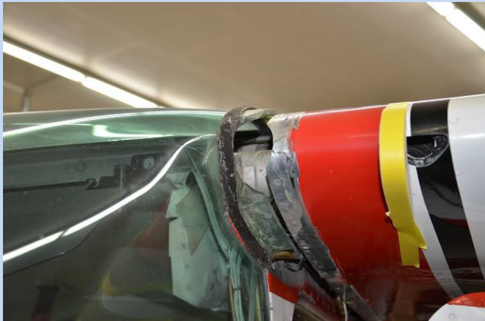
Wing to Fuselage Seals Removed
