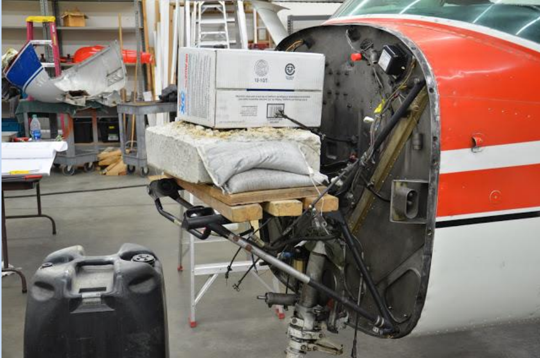
Don't worry...this isn't the new Engine :)... These are weights on the engine mount to keep the Tail off the Ground.
