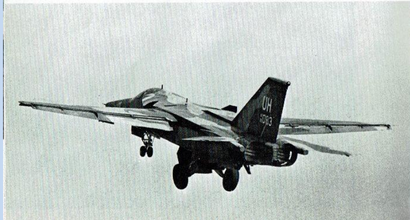
F-111E lifts off with afterburners cooking. The TF-30 engines, which have caused many of the F-111 development problems, were also the first jet engines qualified for supersonic flight at sea level. Their afterburners, unlike conventional turbojet afterburners, are capable of zonal settings. (USAF)
