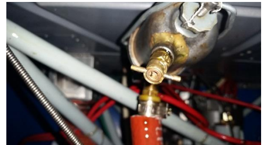
Figure 2: Fuel port, underneath the engine cowling
