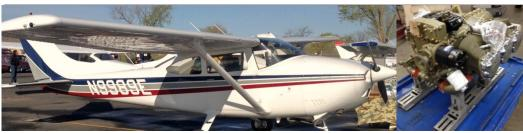
improvements. The basic O-470 engine consisted of two separate configurations identified by the shape and style of the cylinder head. Early models incorporated a parallel valve (also known as a straight valve) cylinder head, large, round intake port and small, two-bolt, exhaust port and stack assembly. The present day standard issue is the angle valve cylinder having a greater cylinder fin area and the induction and exhaust ports with a four bolt pattern.
